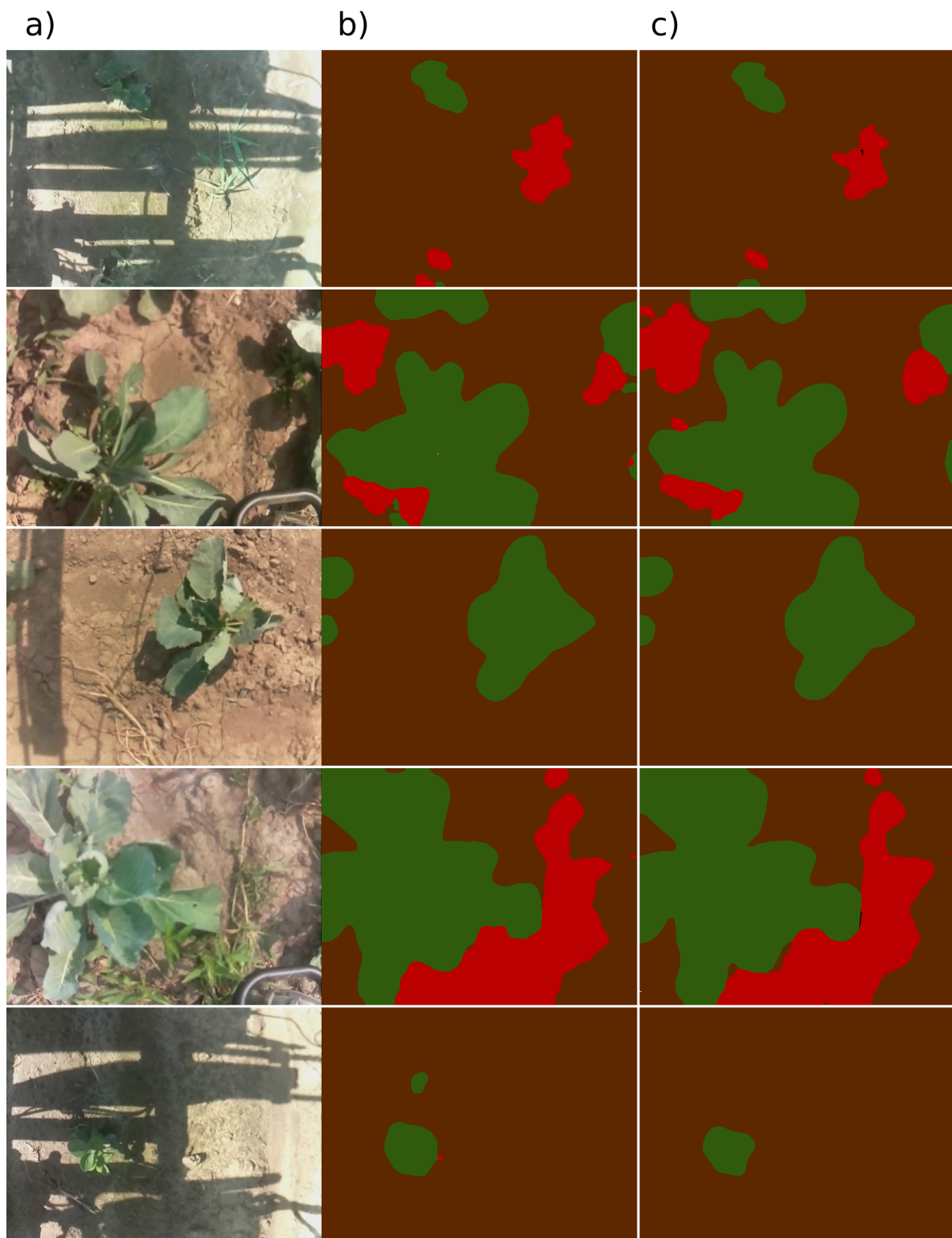
Figure 4. Example predictions of the stationary model: (a) input images (b) segmentation results for a single model instance (c) segmentation results for the ensemble of 50 model instances. Pixels with the highest probability for crops are marked green, weeds are marked red and the ground is marked brown.
