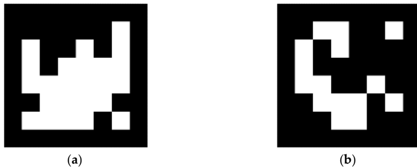
Figure 2. This is ArUco marker: (a) outer marker; (b) inner marker.
