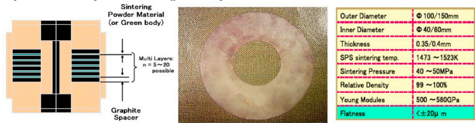
Figure 5. WC/Co sintered very thin plate with a diamond dicing blade [97].
