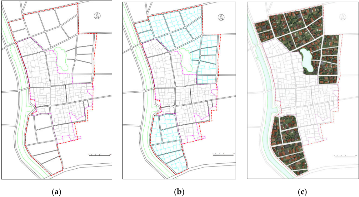
Figure 16. (a) Parameterized automatic generation of the road network; (b) Parameterized automatic generation of the block segmentation; (c) Parameterized automatic generation of the building layout.
