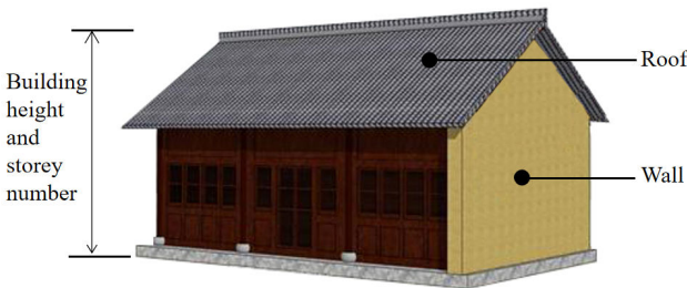
Figure 10. Extracted elements of building facade morphological features.
