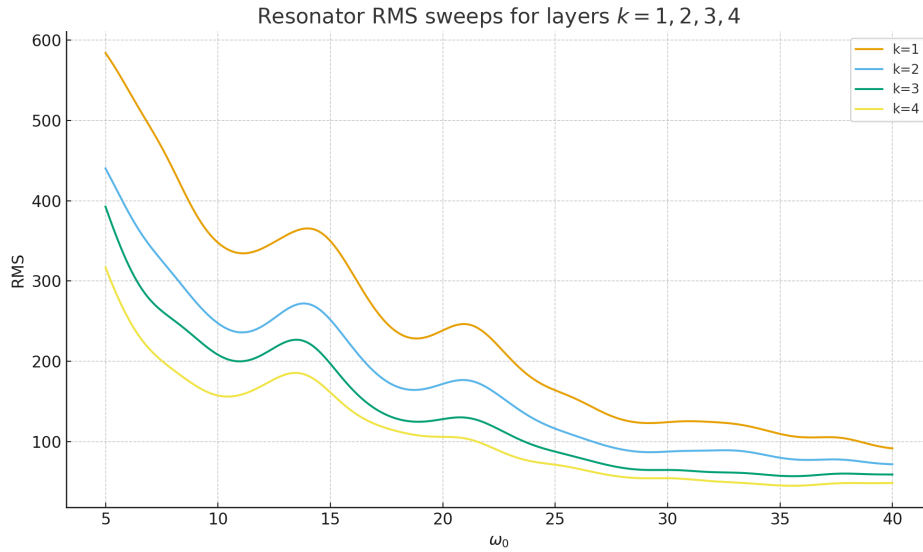
Figure 2. Resonator sweeps \omega_0 \mapsto \text{RMS}_k(\omega_0) for layers k = 1, 2, 3, 4 , obtained by driving a second-order bandpass filter with the windowed signals X_k[j] . The curves share common “hills” at similar values of \omega_0 , while the overall amplitude decreases with k .
