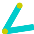
Figure 4. Acrobot environment and goal. A two-link underactuated pendulum in which only the middle elbow joint is actuated. The agent applies a torque u_t to swing the system upward; success occurs once the tip rises above the horizontal target line.
