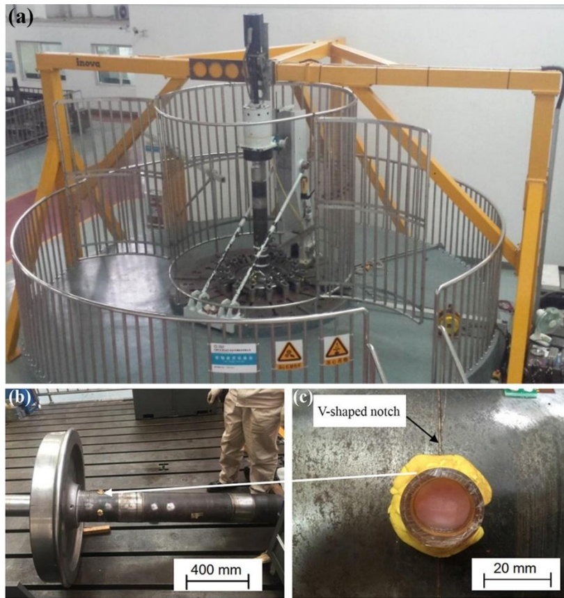
Figure 3. Fatigue test setup and prefabrication of surface notches: (a) the test bench equipped with an experimental high-speed train axle, (b) V-shaped notch on the testing axle, (c) replica sampling of the notch.
