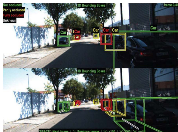
Figure 2. Camera and Lidar 2D fusion for precise distance estimation [9]
