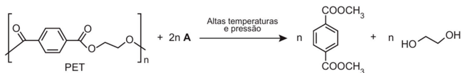
Figure 20. Transesterification of PET: Under high temperature and pressure.
