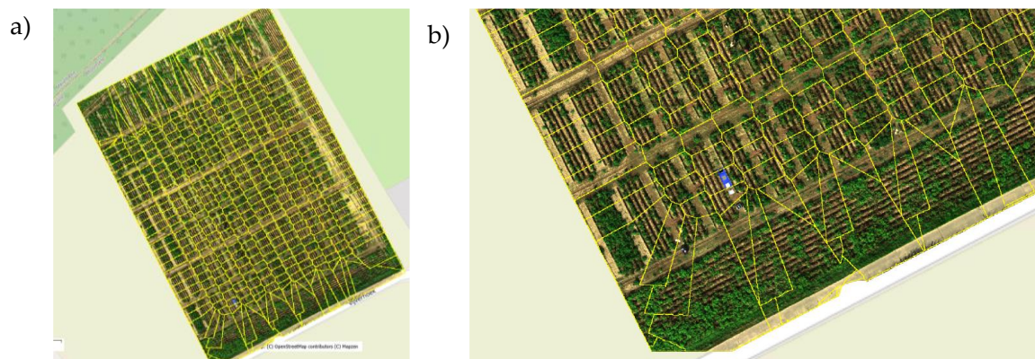
Figure 10. Orthomosaic of a flight generated with a flight overlap of 80% in horizontal and vertical direction. The yellow lines indicate the area taken from each single image. Notice the constant pattern in the core of the images, whereas the edges typically have larger areas from a single image, increasing the risk of anisotropic effects. A) full field; B) detail. Image taken from Agisoft Metashape from a
