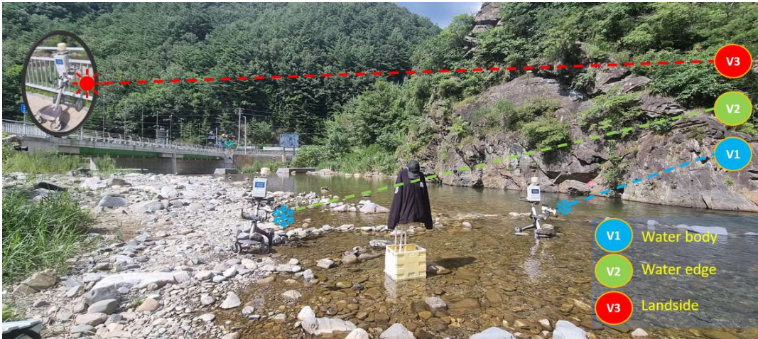
Figure 14. Sensor and AWS Layout (V1: Water Body, V2: Water Edge, V3: Landside).
