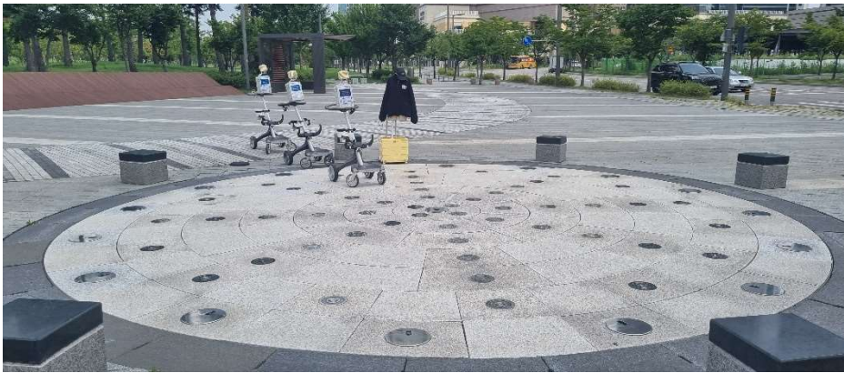
Figure 4. Ground Fountain Sensor Placement (Radius 3.8 m, distances: 2 m, 4 m, 6 m).
