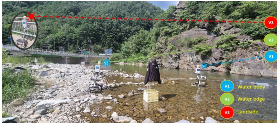
Figure 15. Surface Temperature Sensors for MRT/UTCI at Chilrangi Valley.
