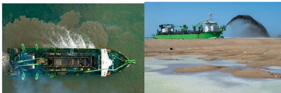
Figure 1. Top view of a dredging vessel (left). View of the rainbowing technique used for sediment disposal (right).
