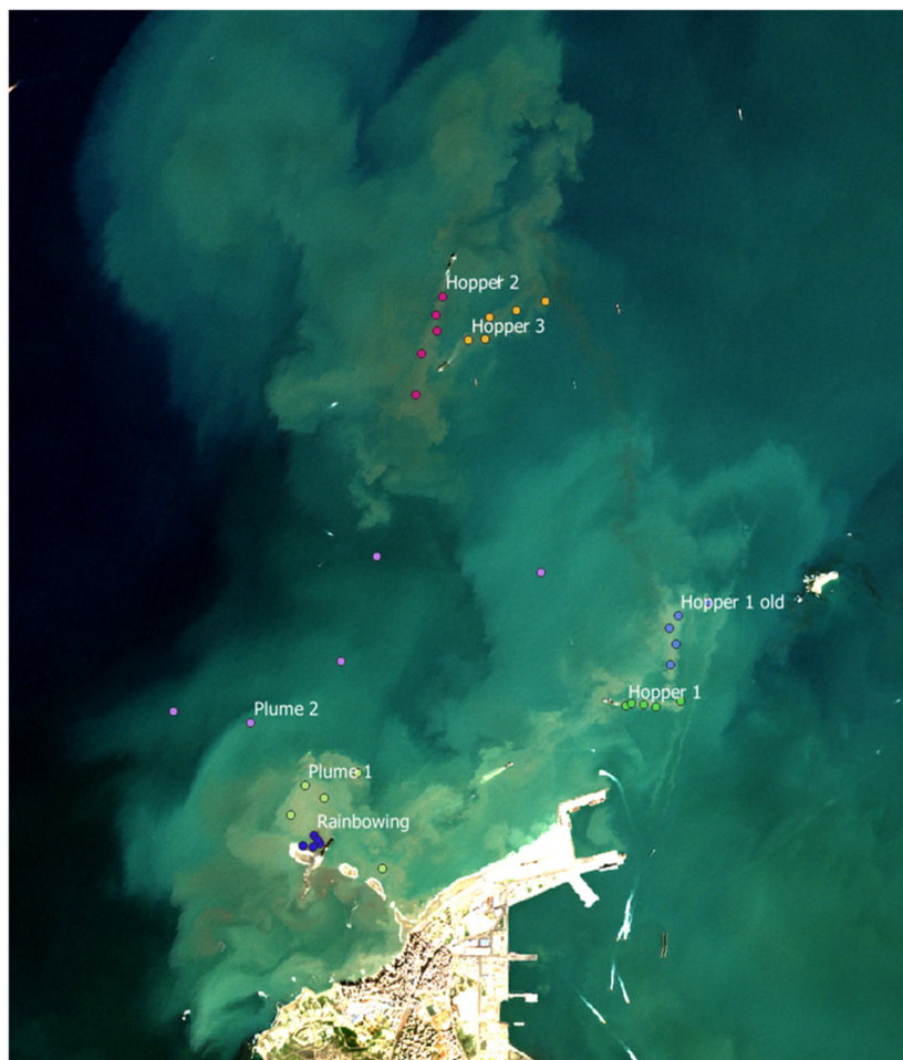
Figure 7. S2 image showing the different hoppers active in the area and the associated dredge plumes.
