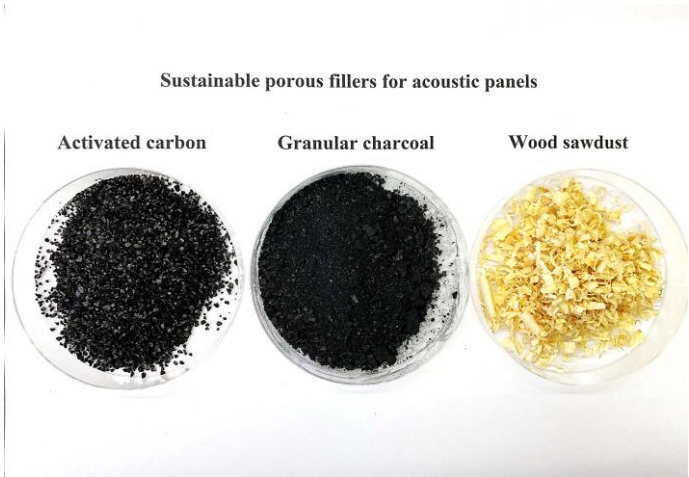
Figure 3. Sustainable porous filler for acoustic panel.
