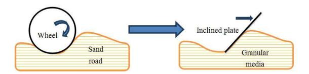
Figure 2 | Wheel effect and its simplified model
