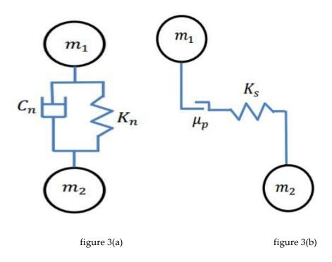
Figure 3 | Contact model in (a) normal and (b) tangential directions
