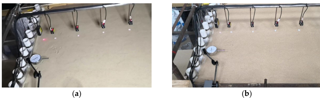
Figure 29. Surface photos of R5 for different excavation depths: (a) The excavation depth is 70 cm; (b) The excavation depth is 80 cm.
