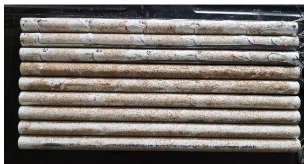
Figure 14. Photo of inclined pile model.
