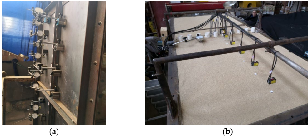
Figure 18. Photos of model after sensor installation: (a) Installation of dial indicator; (b) Installation of laser displacement meter.
