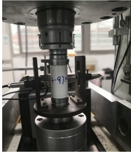
Figure 4. Uniaxial compression test of pile model.
