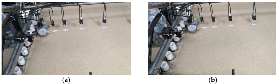
Figure 28. Surface photos of R4 for different excavation depths: (a) The excavation depth is 70 cm; (b) The excavation depth is 80 cm.
