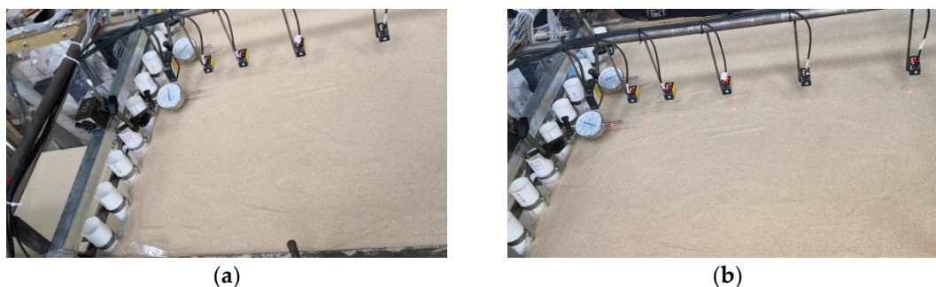
Figure 25. Surface photos of R1 for different excavation depths: (a) The excavation depth is 70 cm; (b) The excavation depth is 80 cm.
