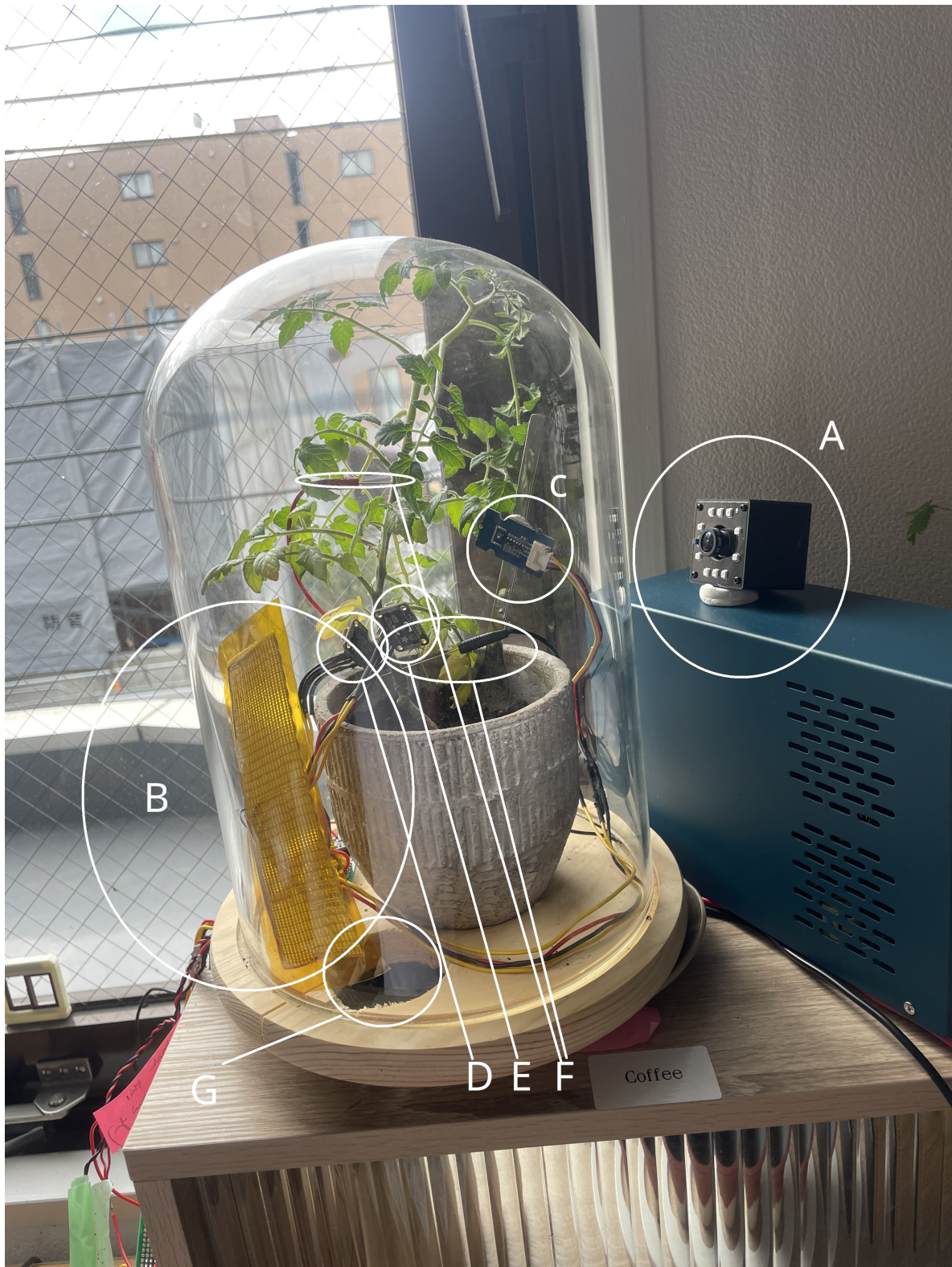
Figure 1. Annotated experimental setup showing sensors, heater, fan and camera positions.
