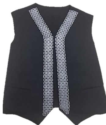
Figure 4. Vest with 3D filaments that can make photovoltaic energy (reproduced with permission) [38].
