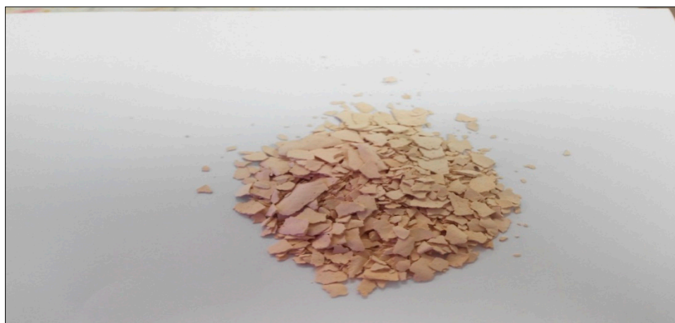
Figure 4.6. Zeolite produced from Spent Bleaching Earth.
