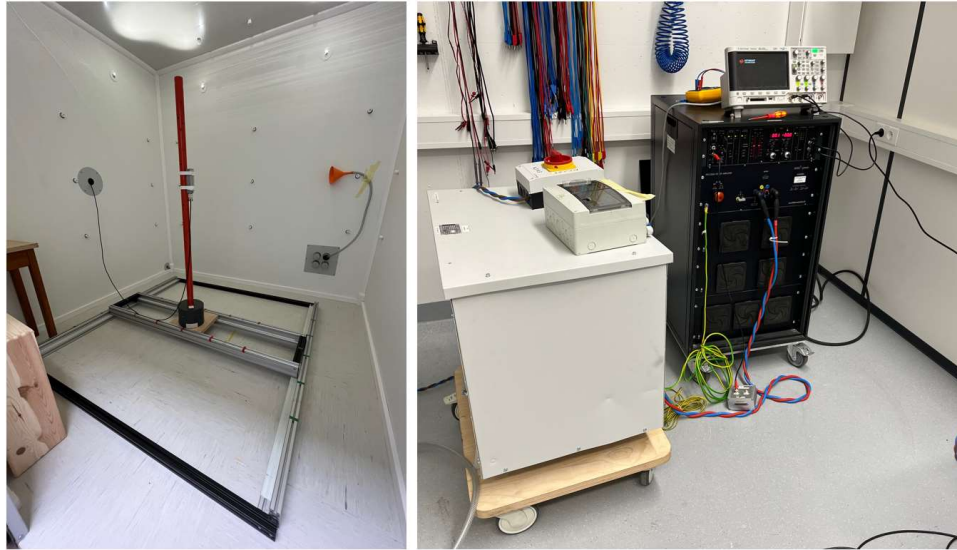
Figure 2. Images of the experimental setup elements. On the left: a picture of the mapping framework using an aluminum rail to adjust the x-y position of the pole, allowing the fluxgate to be positioned at different z-positions. On the right: a photo of the four-quadrant amplifier (black) that drives the degaussing current through the degaussing coil and the transformer (large white box) to eliminate DC offsets.
