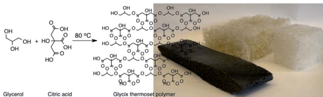
Figure 32. The chemical reaction between glycerol and citric acid gives a 3D thermoset network polymer [59].
