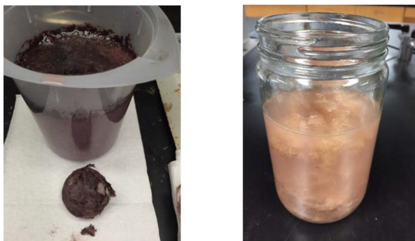
Figure 20. Degraded ball as removed from the reactor after degradation (left ) and after hand-shaking in a container (right) [47].
