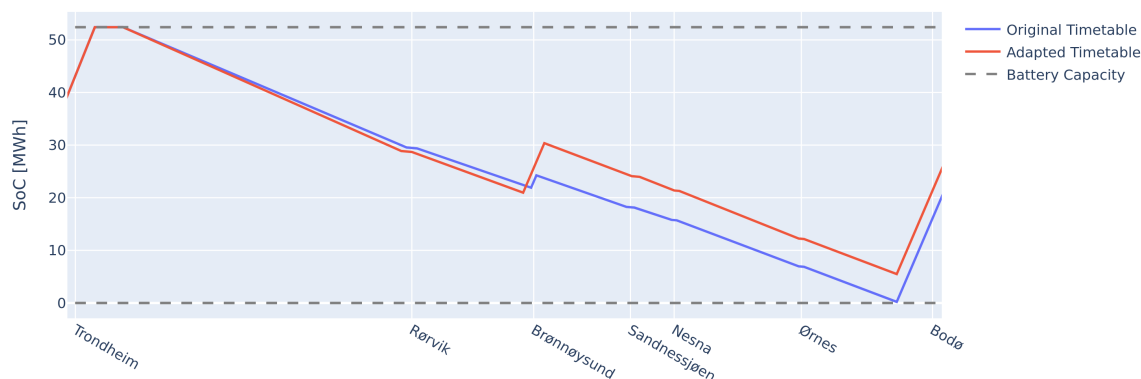
Figure 9. The change in state of charge for the winter-spring timetable and an adapted version.
