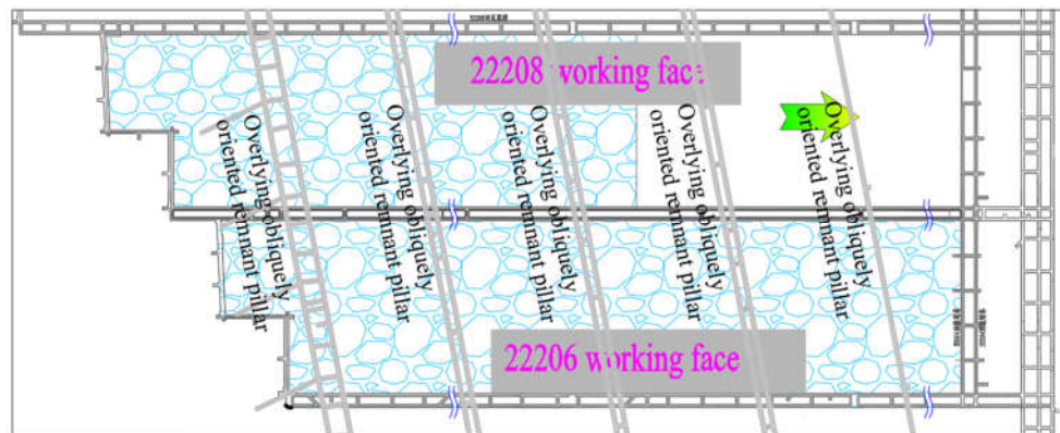
Figure 1 Plan view of the working face and overlying inclined remnant coal pillars.
