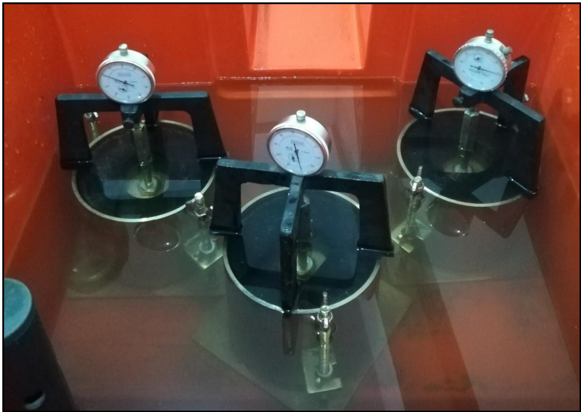
Figure 20. Dial gages placed on top of mold soaked in water for swell measurement after 4 days.
