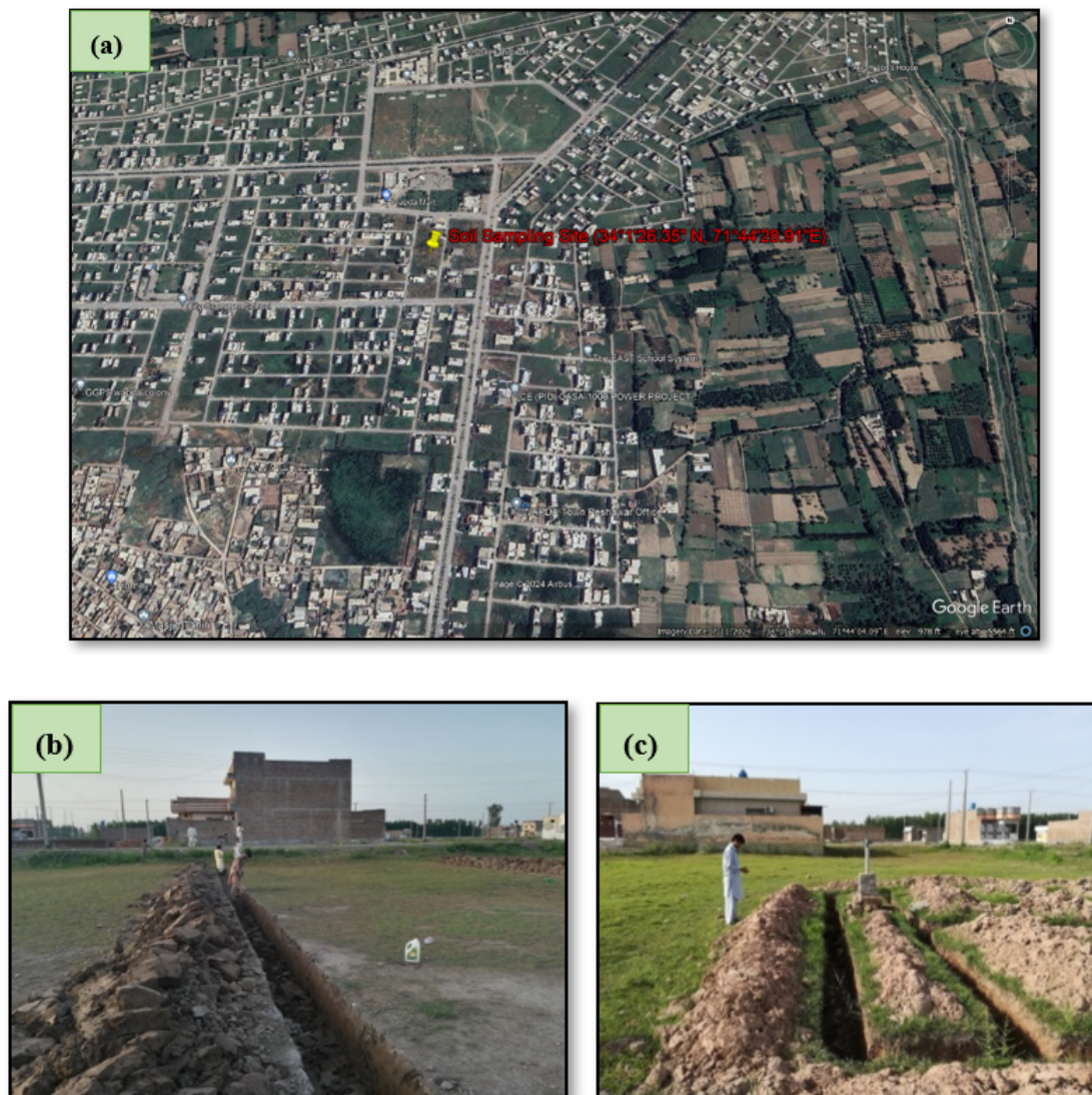
Figure 2. (a) Actual field view of the site; (b) Soil showing desiccation cracks due to wet-dry environment; (c) Pulverized sample.
