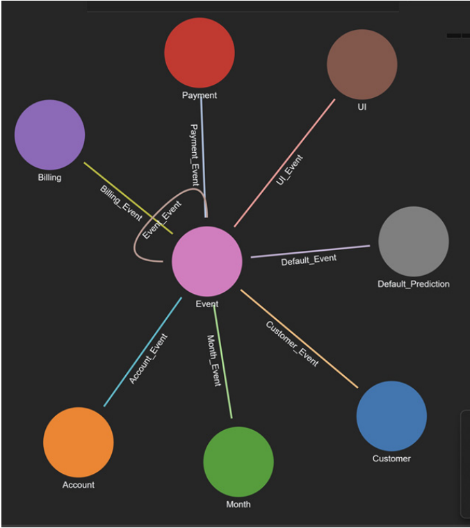
Figure 3. Schema for loan default application services with each node defining a process with inputs and outputs.
