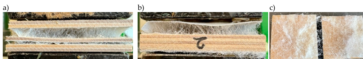
Figure 5. Examples of the tested composites destruction after the internal bond test: (a) plywood 1, (b) plywood 2, (c) the inner surface of the nonwoven fabric layer.
