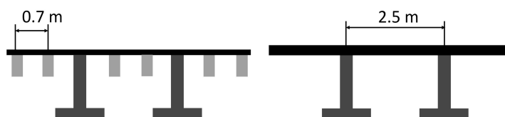
Figure 14. The lumped stiffener simplification principle and its effect on maximum possible mesh size.
