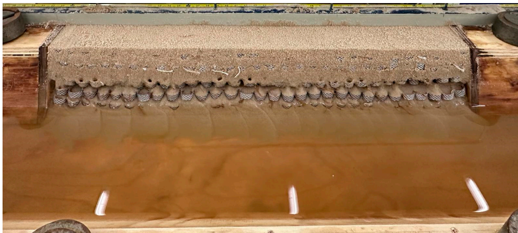
Figure A4. Photos of the reinforced collapsed reinforced embankment at 3L/s.
