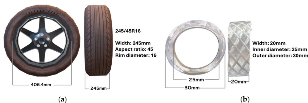
Figure 4. (a) Dimensions of the prototype tyre (Image and dimensions from Tire Size Calculator [40]); (b) the PVC hose model tyre.
