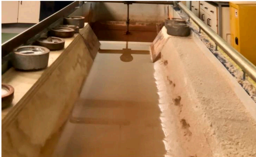
Figure A2. Photos of the collapsed embankment at 3L/s.
