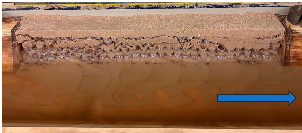
Figure 12. Collapsed reinforced embankment at 7L/s; the arrow represents the direction of the flow.
