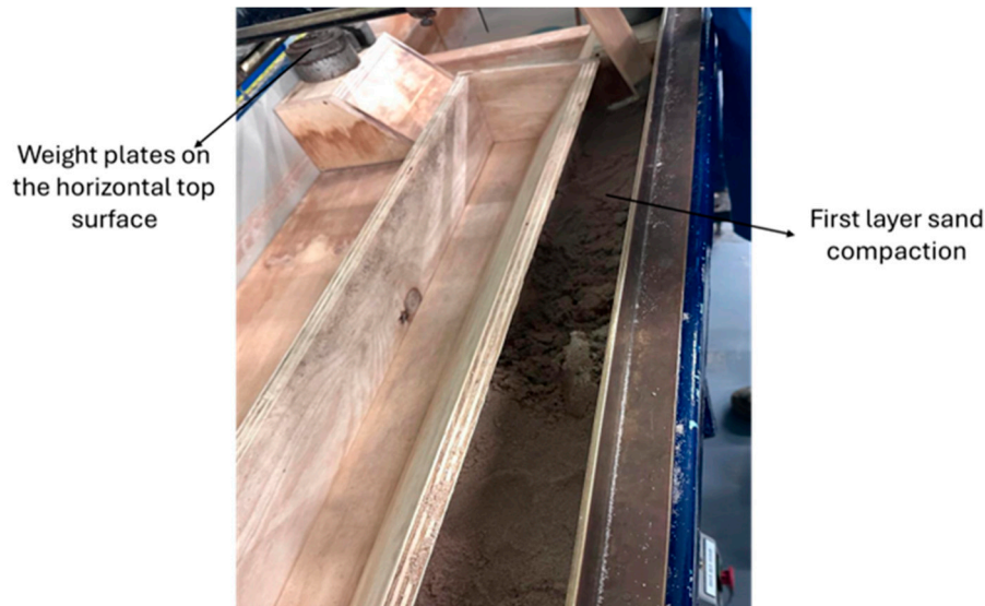
Figure 5. Compaction process of the sand during the construction of non-reinforced embankment.
