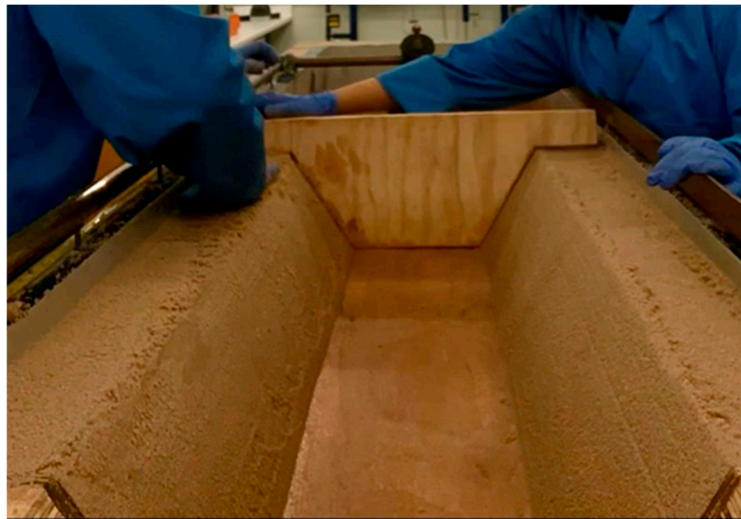
Figure 6. Application of the wooden shaper to finalise the shape of the embankment.
