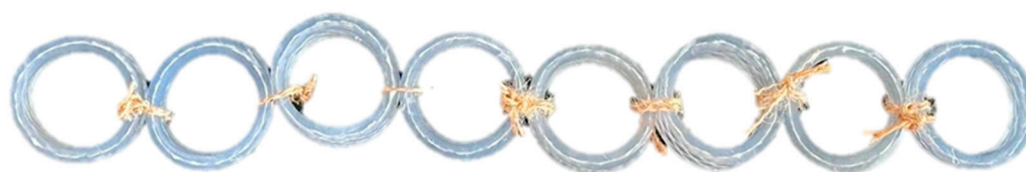
Figure 5. A row of model tyres made of clear PVC hose and tied together using 2mm jute strings.
