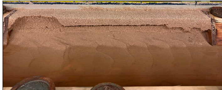
Figure A1. Photos of the collapsed unreinforced embankment at 5L/s.
