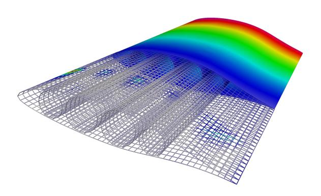
**Figure 1.** Illustrative example of a Wing- Structure- Integrated high-pressure Hydrogen Tanks (SWITHs), similar to APUS i-2 [1].
