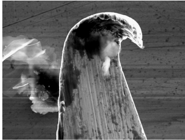
Figure 14. Protruding hook on the needle profile which could cause trauma to the tissues it comes into contact with.
