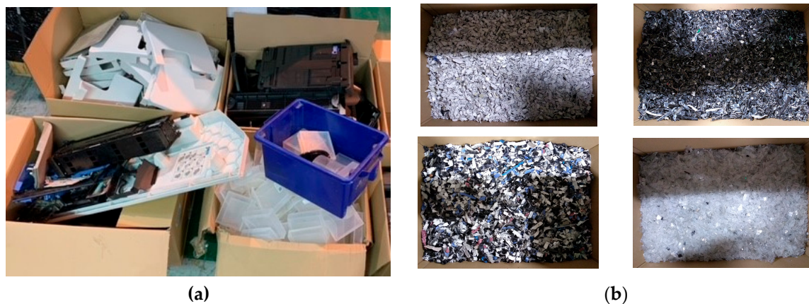
Figure 1. Bulk e-waste plastics identified in the recycling company: (a) raw samples and (b) shredded sample to a particle size to less than 5 mm: white ABS (top-left corner), black ABS (top-right corner), ABS+PC (bottom-left corner), and PP (bottom-right corner).
