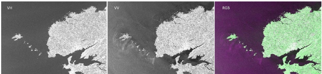
Figure 33. Image acquired by Copernicus Sentinel-1A on 2017/11/01 over Brittany region, France, with VV intensity image, VH intensity image, and RGB color composite. Copernicus Sentinel data (2017) processed by CLS.[87].
