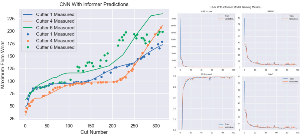
Figure 3.23. One dimensional Convolutional Neural Network - Informer Model for Predicting Tool Wear.
