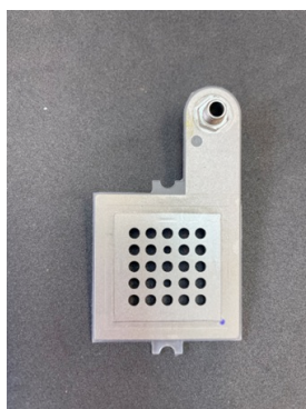
Figure 3. Metal current collector of the fuel cell with a grid geometry.
