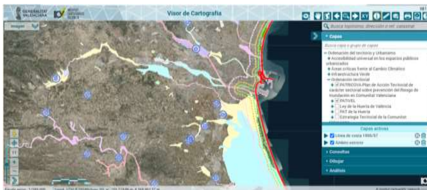
Figure 7. Example of the PATRICOVA cartographic viewer [69]. Screenshot of the digital cartography platform developed by the Generalitat Valenciana, displaying territorial layers related to urban planning, climate change exposure, and coastal dynamics. In addition to fluvial flood risk, the viewer integrates spatial analysis of extreme maritime storm events and the coastal inundation they produce. This tool exemplifies the use of geospatial platforms to support integrated land planning and climate adaptation strategies in vulnerable coastal zones. Source [https://mediambient.gva.es/es/web/planificacion-territorial-e-infraestructura-verde/cartografia-del-patricova].
