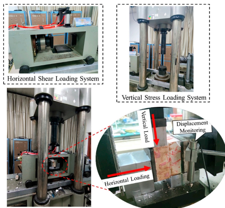
Figure 5. Test system and loading method.
