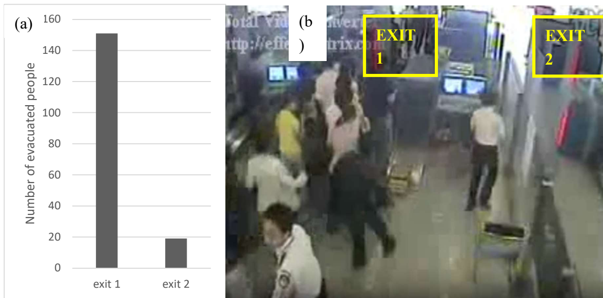
Figure 6. (a) Graph showing the number of people evacuated through exit 1 and exit 2; (b) film still showing the evacuation through exit 1 and exit 2 ( https://ars.els-cdn.com/content/image/1-s2.0-S0378437110008770-mm4.mp4 ) (accessed on 19 January 2025).
