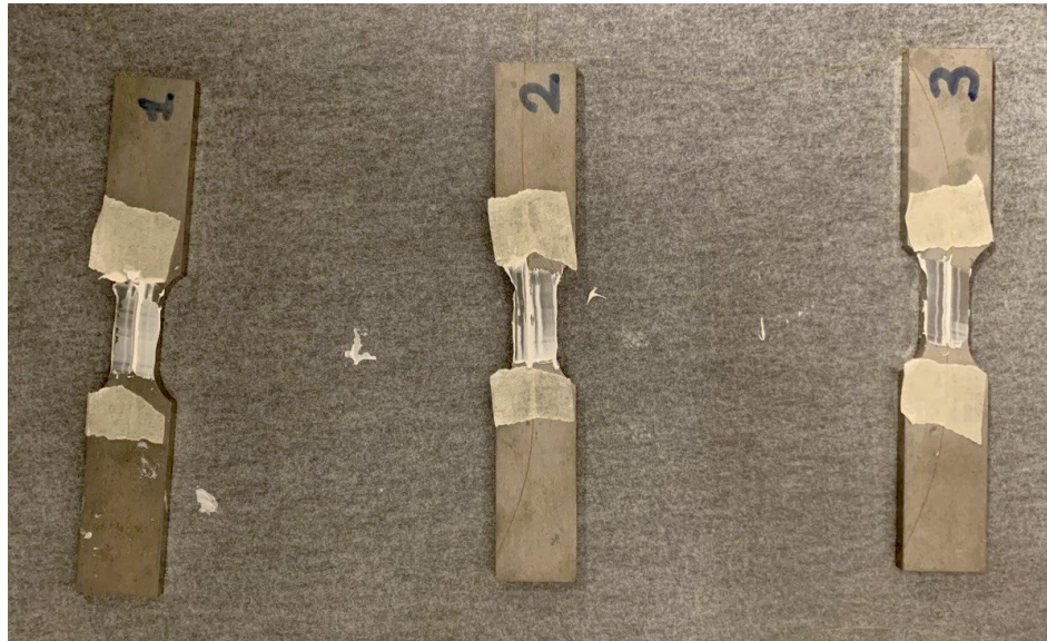
Figure 16. Resin (WEICON Ceramico W) application on the specimens. The FBGs are located at the center of the resin-covered area.
