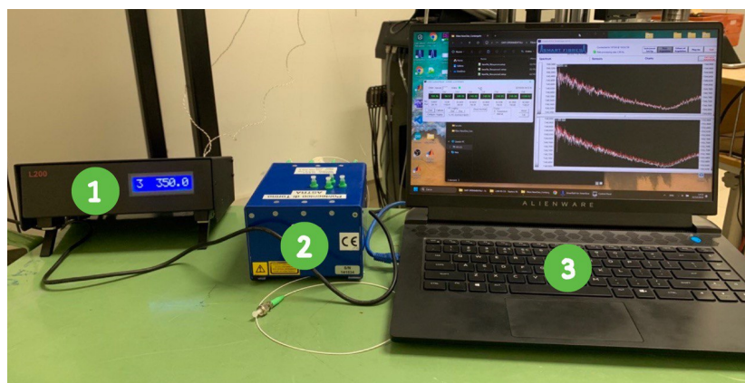
Figure 11. Laboratory setup: (1) Thermocouple reader, (2) SmartScan SBI interrogator, (3) control PC.
