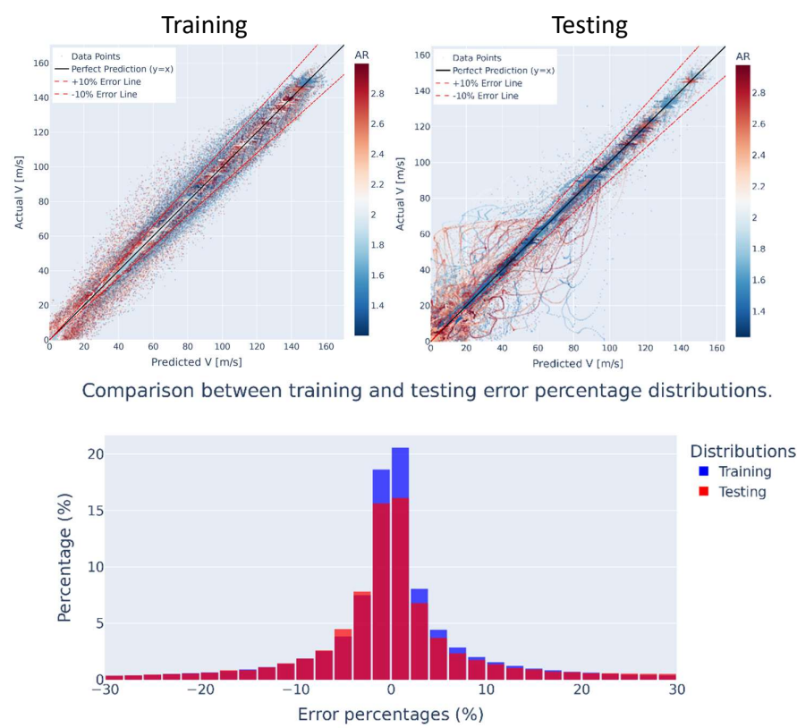
Figure 7. Actual vs. predicted velocities (training and testing) and velocity prediction error distribution (orange colour in figure is the overlapping region).
