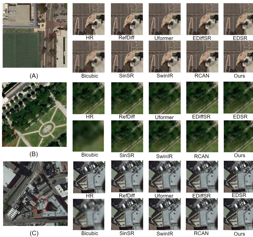
Figure 7. Qualitative comparison at \times 3 scale under blind degradation on the AID dataset. The proposed approach demonstrates superior robustness and detail preservation against complex degradations involving blur and noise.
