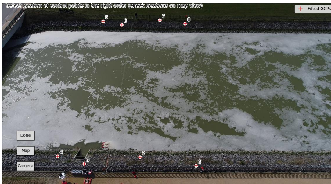
Figure 6. Interface for selecting ground control points.
