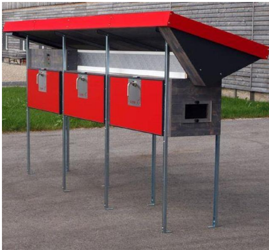
Figure 1. CONA Multifunctional Solar Dryers used for processing Cecropia peltata leaves.
