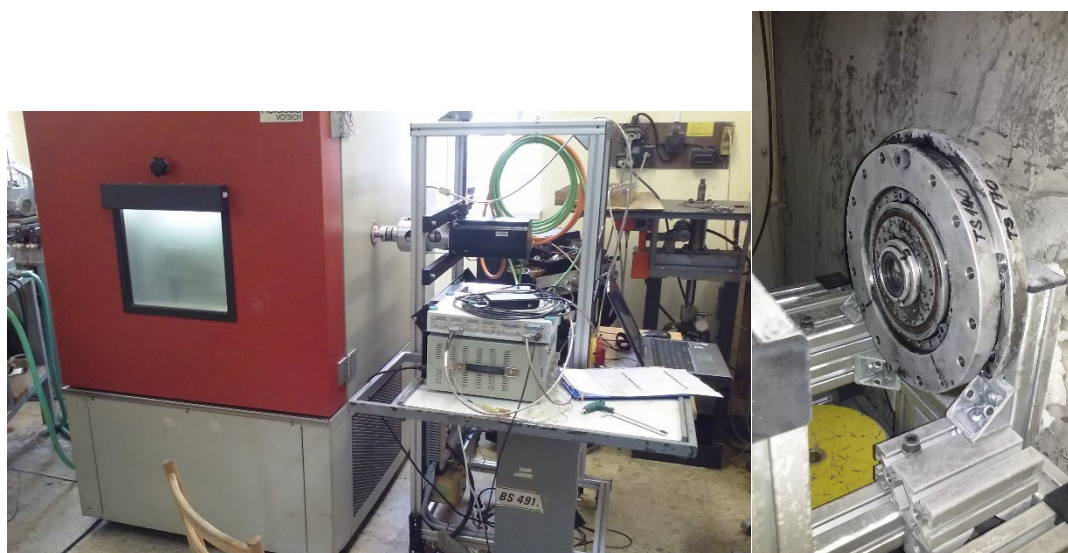
Figure 1. Experimental setup of the TwinSpin TS 140-115-E-P19-0583 cycloidal reducer in the climate chamber.
