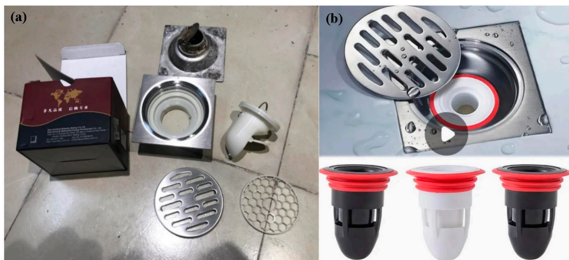
Figure 2. (a) New drain insert with an air valve and magnetic flap. Above is the old drain insert with the air valve stuck in the open position due to corrosion; (b) Inserts with water trap for floor or shower drains.
