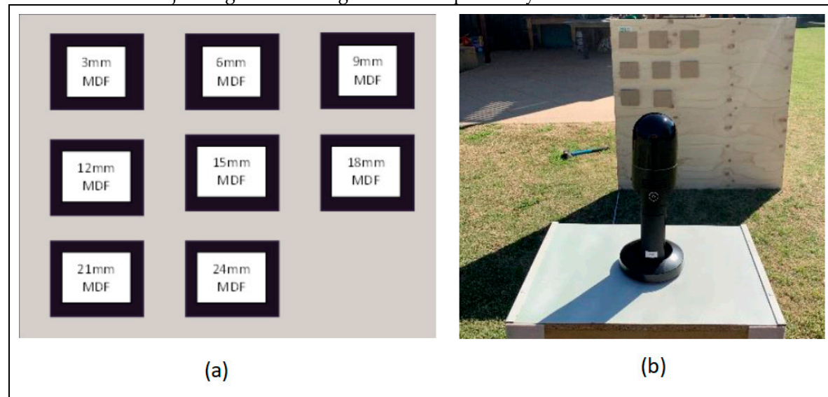
Figure 8. (a) Edge Detection Board; (b) Edge Detection Board with SLAM scanner.
