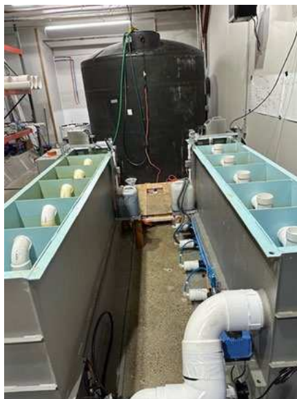
Figure 4. Generation 2 reactor looking towards the water delivery end of the pilot. The 3000-gallon tank in the background is used to fill and transport seater from Puget Sound.
