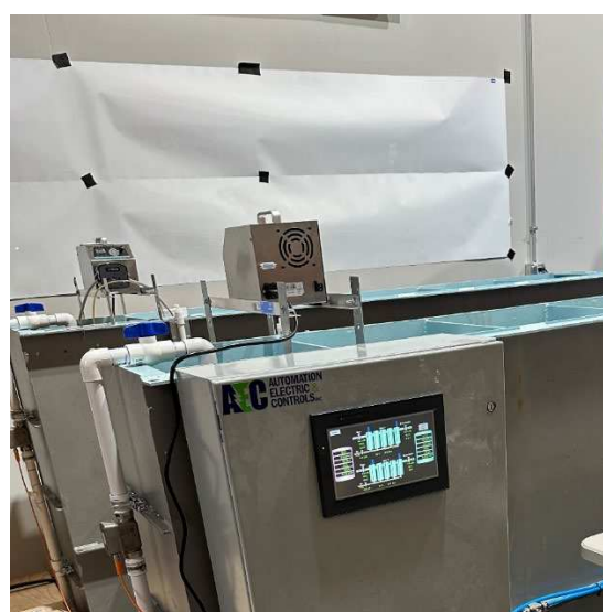
Figure 5. Generation 2 Pilot side view and system PLC. The media pumps sit atop the first reactor cell in each line.
