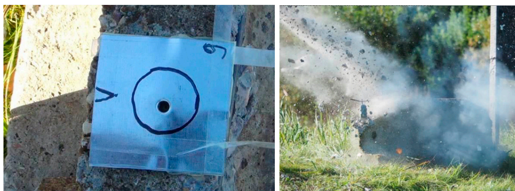
Figure 5. Preliminary investigation of the reaction of 3-picrylamino-1H-1,2,4-triazole (on the left ) to 7.62 mm bullet impact. Control sample of TAGN detonated after bullet impact in a current conditions ( on the right).
