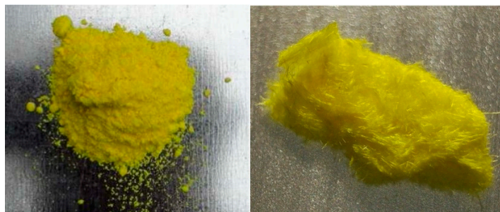
Figure 1. A sample of crystals of 3-picrylamino-1H-1,2,4-triazole after crystallization at 1x (left) and 50x (right) magnifications using a digital microscope.
