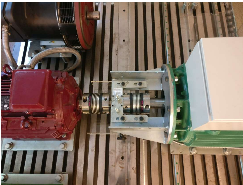
Figure 2. Bellows shaft coupling connects the generator (left) and the motor (right).
