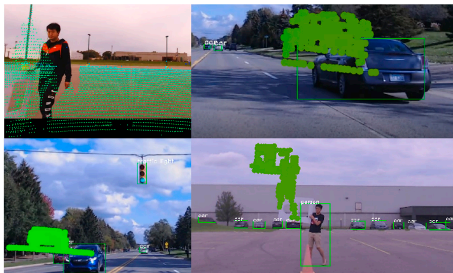
Figure 5. Calibration error results in LiDAR and Camera sensor fusion.
