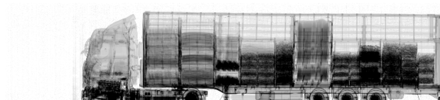
Figure 12. Scan image enhanced using sharpening, histogram equalization, logarithmic transformation, and histogram contrast method.
