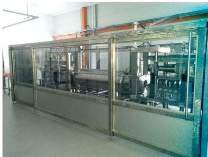
Figure 2. HPP processor with the large volume pressure chamber ( V = 50L ), max pressure P = 600MPa . The central part of the system shows the pressure chamber, and on the right side, there is a mechanism for closing and opening the chamber, as well as for product replacement. It is part of the HPP pilot line in the X-PressMatter Lab of IHPP PAS (Warsaw, Poland). Designed & constructed by UnipressEquipment (IHPP PAS, Poland).
